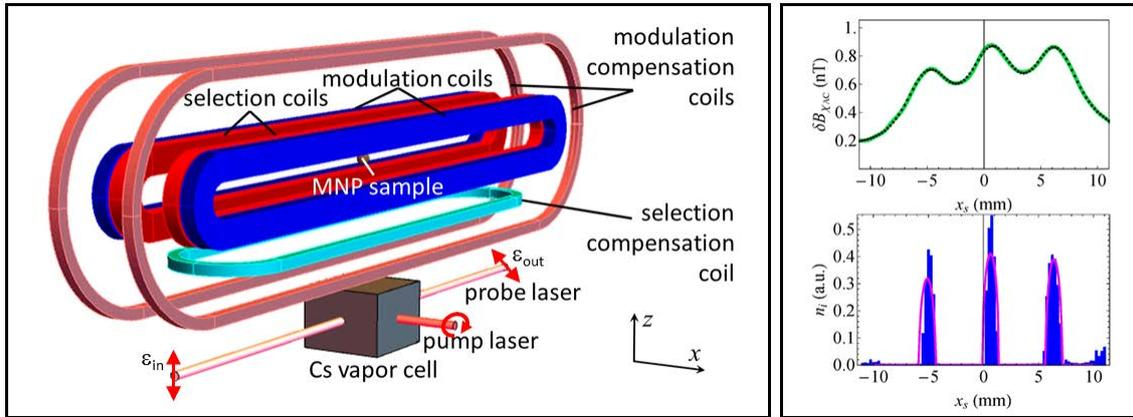
**Fig. 1:** Left: Sketch of the experimental set-up for performing MPI measurements on MNPs with a Cs AM. Right: Example of a 1D MPI scan of a structured MNP sample (top) and deconvoluted MNP density distribution (bottom).
