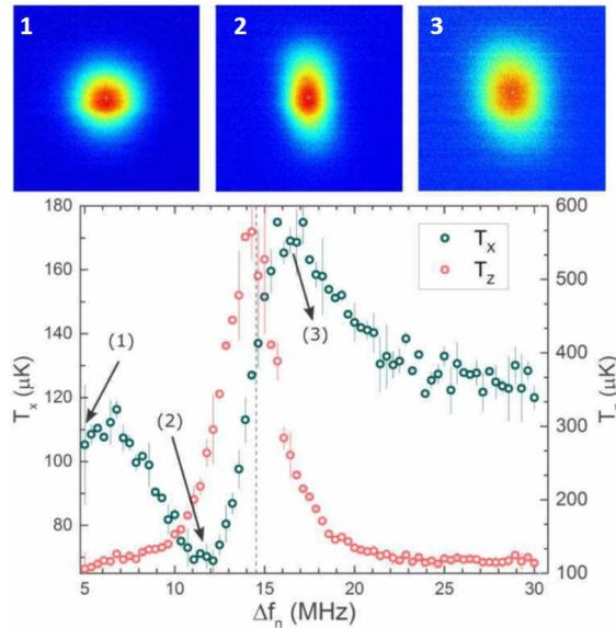
Fig. 1: Temperature obtained by TOF spectroscopy after 1D FC cooling as a function of FC detuning
