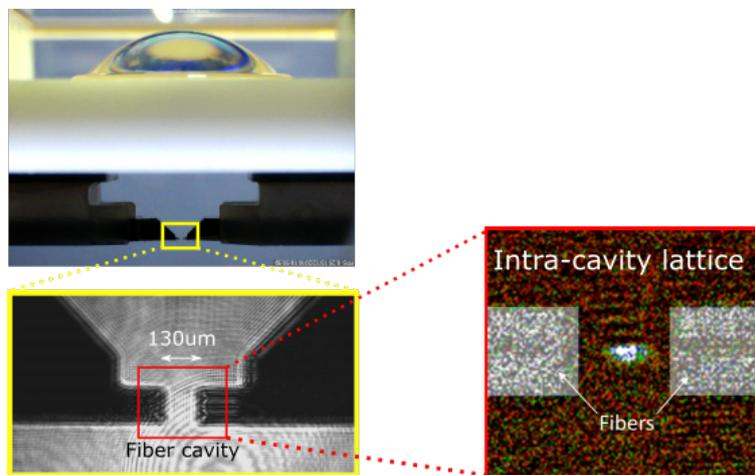
**Fig. 1:** Optical image of the heart of the all-in-vacuum experiment. The fiber Fabry-Perot cavity (first inset) is placed at the focus of a high-numerical aperture lens. The second inset shows an absorption image of 2000 trapped atoms in the cavity lattice.
