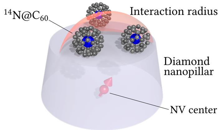
**Fig. 1:** Schematic of a diamond nanopillar ( $r \sim 100$  nm) containing a single nitrogen-vacancy color center which is coupled to few N@C<sub>60</sub> spin qubits on the surface (image not to scale).
