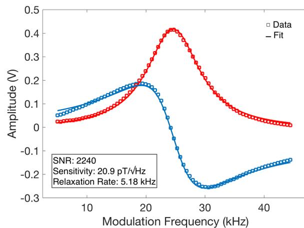
**Fig. 1:** Measured data and fits to the in-phase and quadrature components of the magnetic resonance signal. A 300 nT RF modulation field is applied across a range of frequencies and a resonant response observed in the presence of a 7  $\mu$ T static field.
