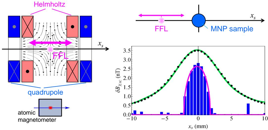
**Fig. 1:** Left: Principle of 1D-MPI scanner with gradient and homogenous field coils producing a field-free line (FFL), whose position can be moved along the  $x_s$  axis by scanning the the Helmholtz coil current (compensation coils [5] not shown). Right: Raw magnetometer signal (green line) from a cylindrical 4 mm diameter MNP sample, and inferred 1D MNP density distribution (blue histogram) and reconstructed signal (black dots).
